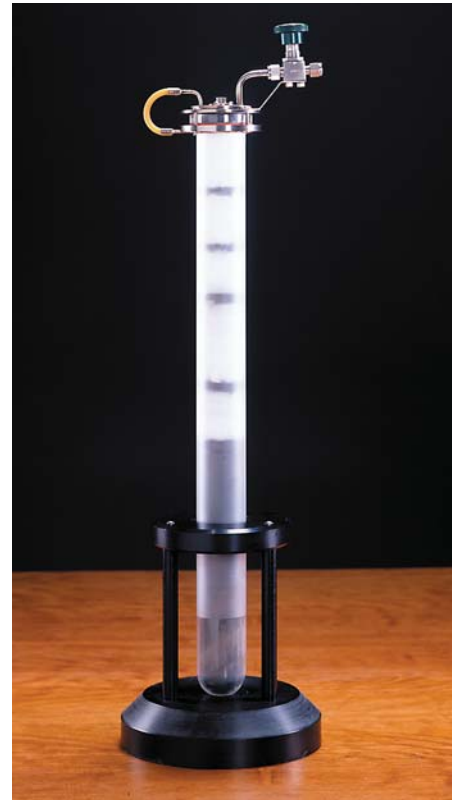
Open cells allow users to minimize the uncertainty from pressure corrections by regulating cell pressures themselves.
