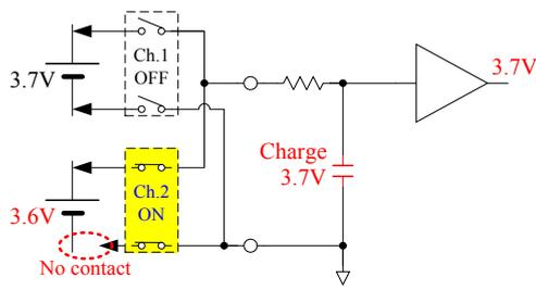
Fig. 7 During measurement of Ch. 1 (normal)
