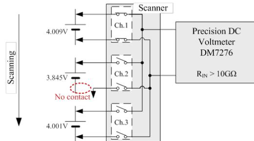
Fig. 9 Scan measurement connection diagram
