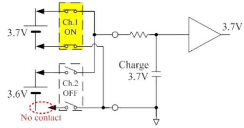
Fig. 8 During measurement of Ch. 2 (no test probe contact)
