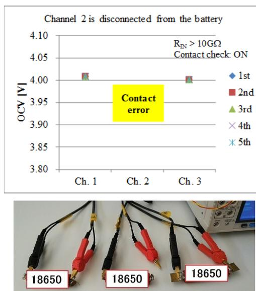
Fig. 12 Measurement with Ch. 2 left open and the DC voltmeter's contact check function enabled
