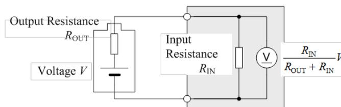
Fig. 4 Voltage source output resistance and measured values
