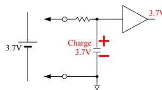
Fig. 6 Residual charge of capacitor
