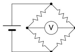
Fig. 2 Measurement of a strain gauge
