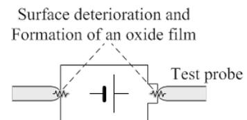
Fig. 3 Test probe contact
