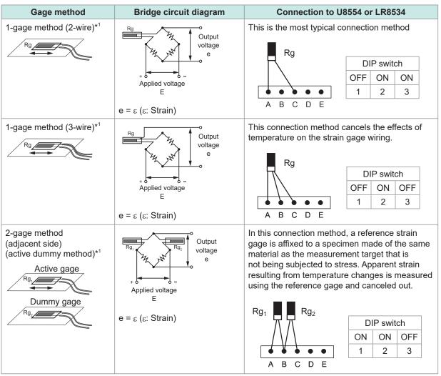
\*1: Must be corrected using (1,000,000 × measured value) / (1,000,000 - measured value). The scaling function cannot be used to perform correction. Instead, perform correction using the waveform calculation function.
