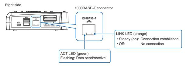
The LINK LED will light up when the instrument has connected to the network, indicating that the connection can be used. If the LED fails to illuminate, there may be a malfunction of the instrument or connected device or a wire break in the LAN cable.
