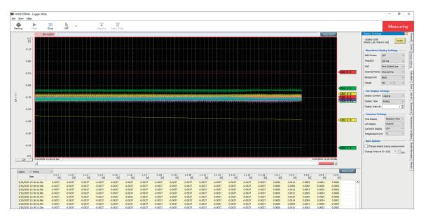
When a recording interval of between 1 ms and 5 ms is set, the system cannot acquire data in real-time
