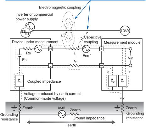
Other device's leakage current or earth current that flows due to difference in grounding potentials
