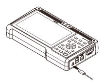
Insert the USB cable's plug into the instrument's USB cable connector, exercising care to ensure that the plug is oriented properly.
