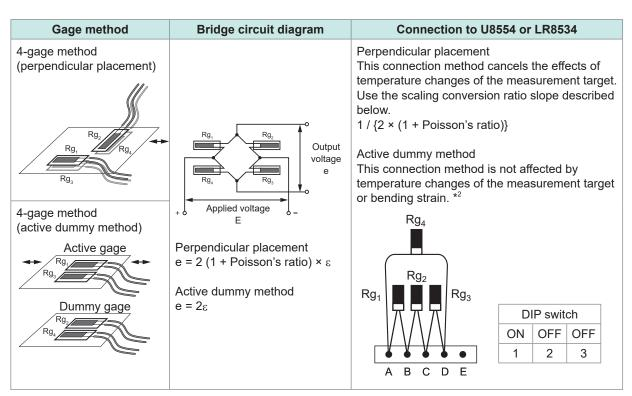
\*2: Must be corrected using (2,000,000 × measured value) / (4,000,000 - 2 × measured value). The scaling function cannot be used to perform correction. Instead, perform correction using the waveform calculation function.
