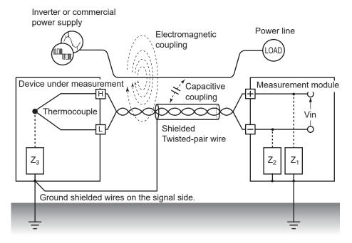
Keep signal lines (thermocouples) away from wires that could serve as sources of noise (power supply lines, etc.). Furthermore, you can block capacitive coupling by shielding and grounding signal lines.
