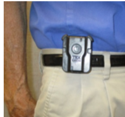
The NEON tracking unit contains a gyroscope, accelerometer, barometric pressure sensor, compass, and ranging sensors.
