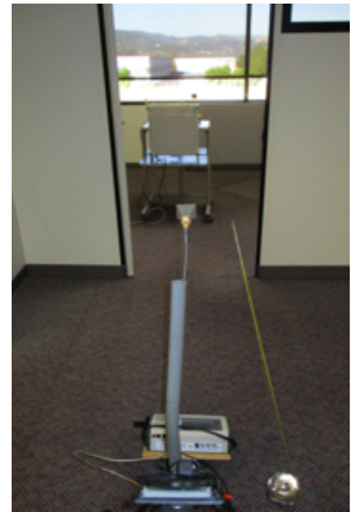
Anritsu MS2720T Spectrum Analyzer (on a cart) with flexible cable and 26.5 to 40 GHz waveguide to coax adapter and 10 dB gain horn antenna.
