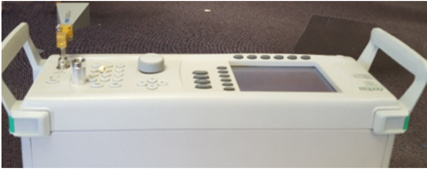
Anritsu MG3694C signal generator providing a +12 dBm signal into a 26.5 to 40 GHz waveguide to coax adapter and 10 dB gain waveguide horn antenna.
