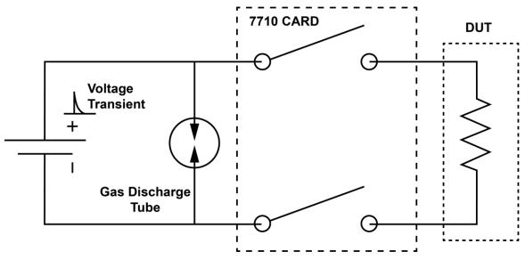
If the device under test (DUT) changes impedance states during testing, excessive currents or voltages may appear at the solid state relay. If a DUT fails due to low impedance, current limiting may be required. If a DUT fails due to high impedance, voltage clamping may be required.
