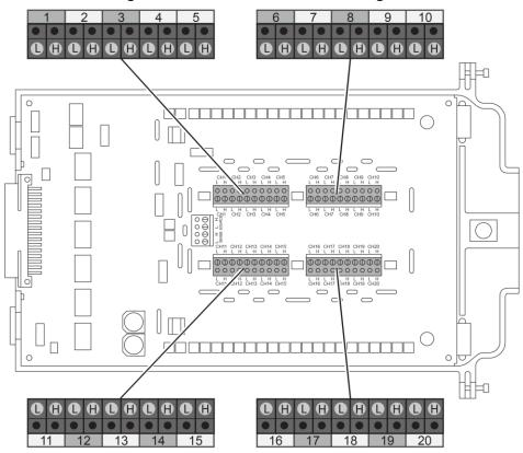
Figure 4: Screw terminal channel designations
