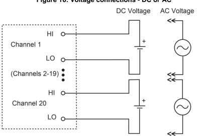
Figure 10: Voltage connections - DC or AC
