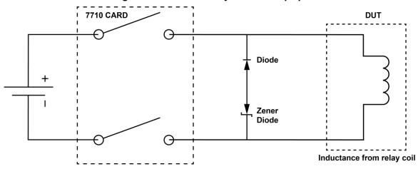
Figure 14: Diodes at relay coil to clamp spikes
