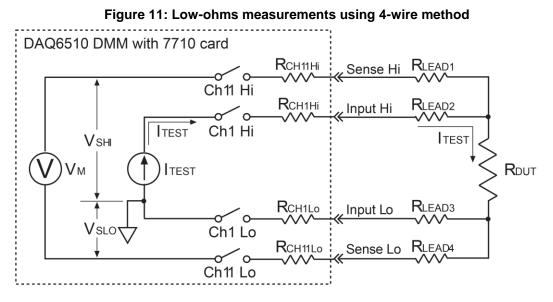
Assumptions: Virtually no current flows in the high-impedance sense circuit due to the high impedance of the voltmeter (VM). Therefore, the voltage drops across Channel 11 and test leads 1 and 4 are negligible and can be ignored.
