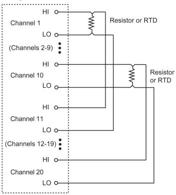
Figure 9: Four-wire resistance and RTD connections
