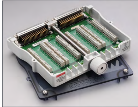
3720-ST: Screw Terminal Block. Required with the 3720 for automatic CJC thermocouple measurements.
