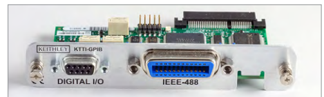
KTTI-GPIB GPIB interface with 6 digital I/O ports.
