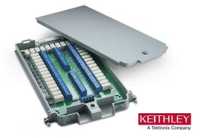
The 7708 plug-in module offers 40 channels of 2-pole or 20 channels of 4-pole multiplexer switching that can be configured as two independent banks of multiplexers. The built-in CJC sensors automatically linearize thermocouples, making the 7708 ideal for RTD, thermistor, and thermocouple temperature applications. It is also well suited for mixed-signal measurement applications that require multi-point monitoring, such as environmental stress screening.
