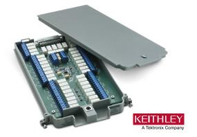
The 7702 plug-in module offers 40 channels of 2-pole or 20 channels of 4-pole multiplexer switching that can be configured as two independent banks of multiplexers. The 7702 provides two additional protected channels for current measurements. It is ideal for RTD, thermistor, and thermocouple temperature applications.
