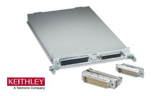
The 7701 plug-in module offers 32 channels of 2-pole or 16 channels of 4-pole multiplexer switching. Its 32 channels can be configured for common-side 4-wire ohms. They can also be configured as two independent banks of multiplexers. It is ideal for RTD or thermistor temperature applications.
