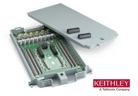
The 7710 plug-in module offers 20 channels of 2-pole or 10 channels of 4-pole relay input that can be configured as two independent banks of multiplexers. The relays are solid state, providing long life and low maintenance. Solid-state relays usually have 100 times longer life than mechanical relays. It is ideal for long-term data logging applications as well as for demanding high-speed applications.
