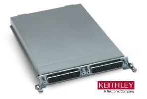
The 7703 plug-in module offers 32 channels of 2-pole or 16 channels of 4-pole multiplexer switching that can be configured as two independent banks of multiplexers. The non-latching reed relays provide high speeds and are designed for 300 volt, 500 mA; 10 VA. The relay closures are stored in onboard memory. The 7703 is ideal for RTD and thermistor temperature applications.
