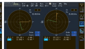
Harmonic two-circuit vector display
