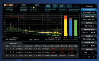
Use the scan table to set up frequency ranges, gains, bandwidths, and dwell time
