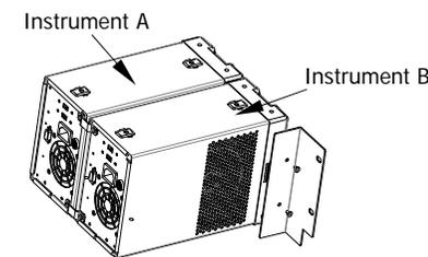
10. Attach the filler panel to the right side of Instrument A, then secure it with two M4 pan head screws.
