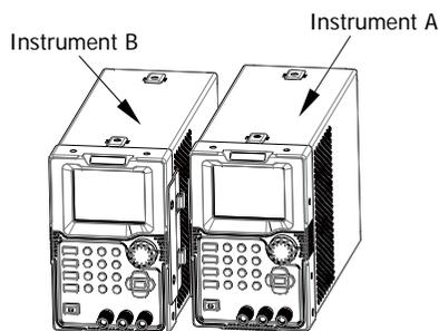
8. Place two retaining brackets onto the connecting positions of the rear panels of the two instruments, and then secure the retaining brackets with four M4 pan head screws.
