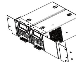
12. Place the assembled instruments and rack onto the bottom plate. Then, secure the left and right fasteners to the cabinet by using four M6 screws and four M6 nuts.
