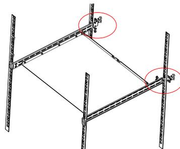
6. Attach Connecting Plate A to the left side of Instrument A and attach Connecting Plate B to the right side of Instrument B, then secure them with four M4 countersunk flat head screws.
