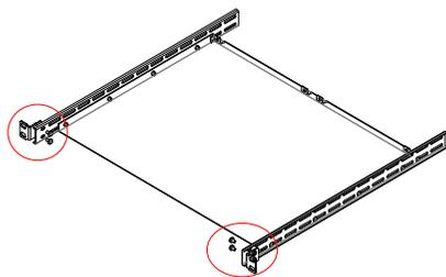
4. Secure the side beam fasteners to the cabinet by using four M6 screws and four M6 nuts.
