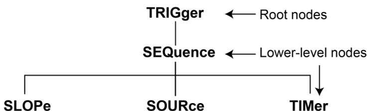
You can create commands and queries from these subsystem hierarchy trees. Commands specify actions for the instrument to perform. Queries return measurement data and information about parameter settings.
