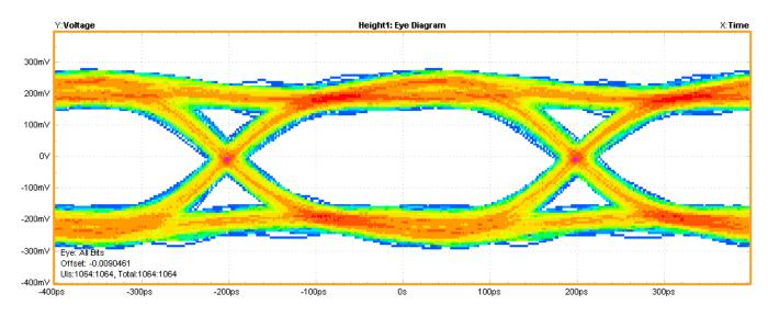
FIGURE 8. Eye diagram used in HS-TX Clock-to-Data-Lane timing test.
