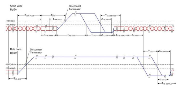
FIGURE 5. Modes and States in a D-PHY clock lane in normal clock mode. (MIPI Alliance Specification for D-PHY, Version 1.2, MIPI Alliance, Inc.)
