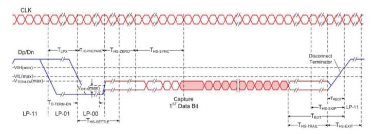
FIGURE 4. Modes and states in a D-PHY data lane in continuous clock mode. (MIPI Alliance Specification for D-PHY, Version 1.2, MIPI Alliance, Inc.)
