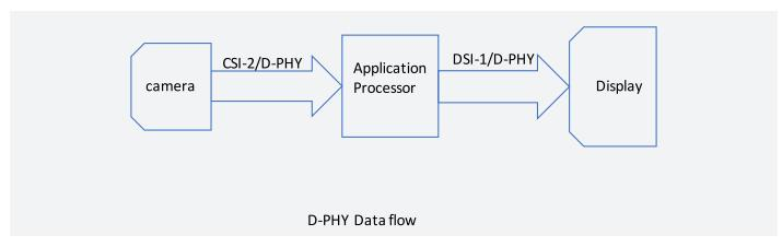
FIGURE 2. The D-PHY physical layer can support different protocols to optimize data transfer.
