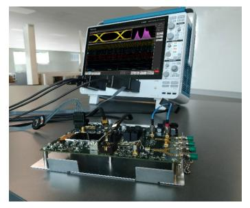
FIGURE 1. 6 Series MSO oscilloscope with high-bandwidth TriMode probes provide a solid foundation for automated compliance testing.
