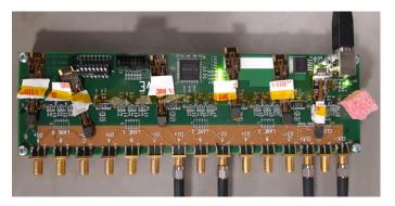
FIGURE 7. D-PHY termination board, with TriMode probes soldered in place.
