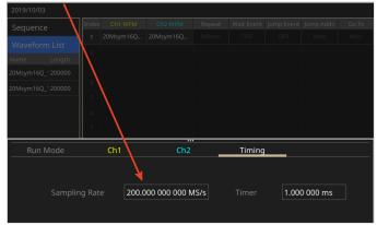
To run these waveforms, hit the Ch1 and Ch2 "On" keys, then hit the Run key on the front panel. Note that any changes in the Settings Bar menu will only take effect after toggling the Run key off and on again.
