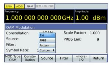
To create the output, simply hit the **RF** and **Mod ON/OFF** keys (translucent). They will illuminate when active.
