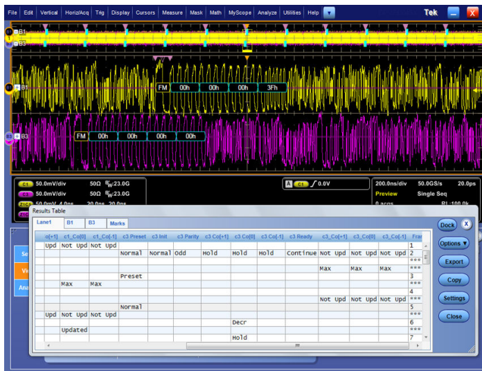
Link Training (option HSSLTA) - Offers an interactive Results Table based on FastFrame records. - Fast-Frame Records: Time-aligned Hex and Bit-level decode, Marks (Frame, Control Channel, and Training Data). Results Table: All negotiation data is captured in Results Table, Click row to view waveform, Scroll through table rows, Verify Negotiation Requests/Responses, and Export Negotiation Data.
