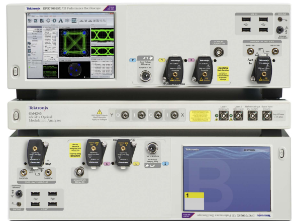
DPO7000SX units may even be operated inverted if desired, to shorten OMA receiver connection distance as shown.
