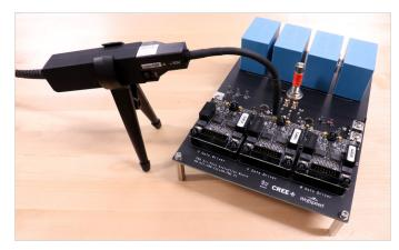
Figure 12. MMCX connectors - Example 1. Photo Wolfspeed. Reprinted with permission.
