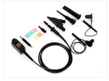
Figure 5. Tektronix TPP0850 Voltage Probe. Single-ended, ground-referenced probe with 50× attenuation (up to  $100V_{\rm RMS})$  and 800 MHz bandwidth.
