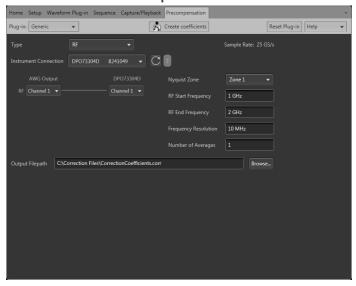
The Tektronix Generic Precompensation application plug-in enhances the capabilities of either the AWG70000A Series Arbitrary Waveform Generators or the SourceXpress® waveform generation software, adding the ability to create correction coefficients that can be applied on waveforms to get flat frequency and linear phase response.
