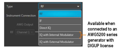
As you choose the different Types, the available settings change along with an illustration of the connections that must be made between the arbitrary waveform generator output and the instrument being used to capture the resulting signal.
