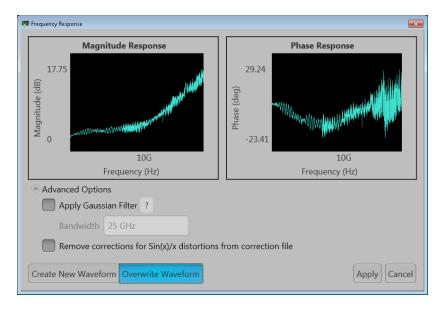
Choose to either create a new waveform or overwrite the existing waveform. (For RF type corrections, you also have the Advanced options to apply a Gaussian filter or remove Sin(x)/x distortions.
