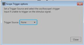
Triggering with the stimulus signal may result in triggering problems due to trigger bandwidth limitations. In these instances, you may want to trigger the oscilloscope with the AWG marker signal or provide an external trigger signal.
