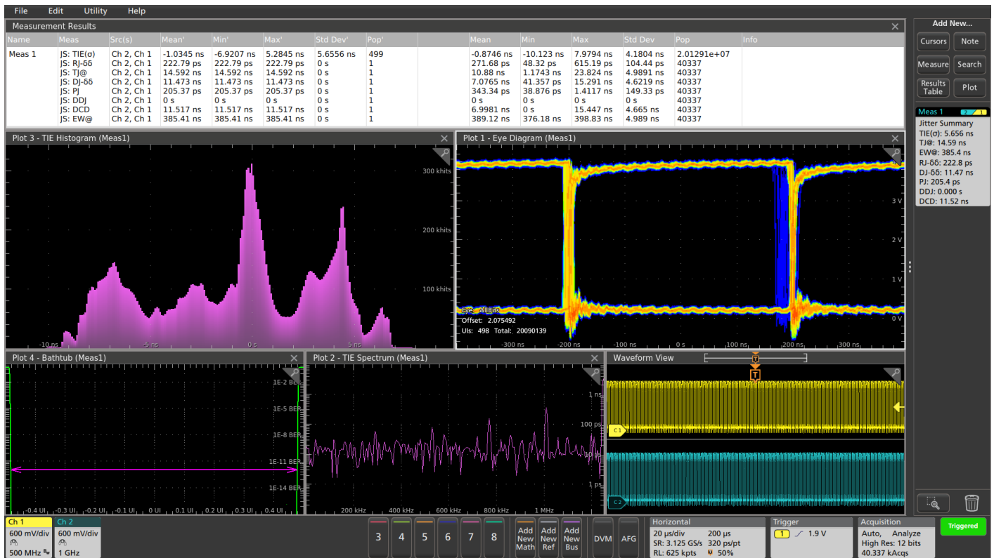
FIGURE 10. Jitter analysis of a synchronous logic circuit.
