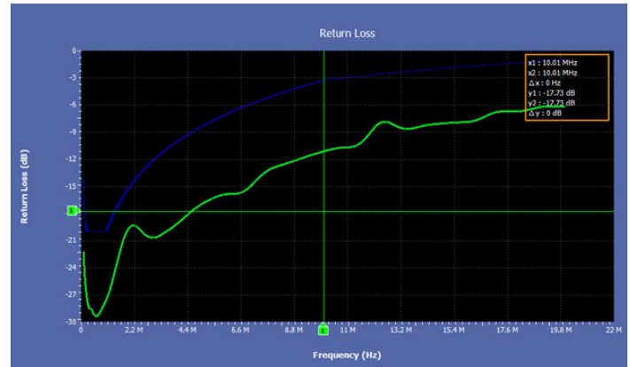
Return loss plot generated using oscilloscope and AWG method
