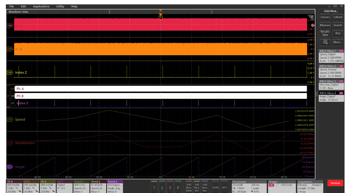
Measuring motor speed and direction using QEI method. The QEI signals (Phase A, B, and Z index) are shown for reference by connecting both Analog (TPP1000) and Digital (TLP058) probes.
