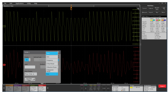
Add and configure the Time Trend plot on different sub-measurements of Power Quality measurement. The image shows two time-trend plots monitoring Vrms and Frequency parameters.
