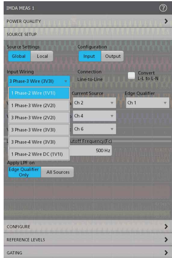
Configuring the measurement for Input wiring configuration
