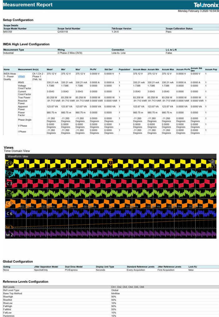
A sample IMDA test report file with summary, details, and corresponding images
