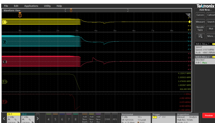
Time trend plot displaying deceleration of a motor into a stop state
