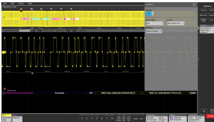
Automated search in wave inspector finds all specified bus elements. The image displays the 6 start-of-frame events in the acquisition.
