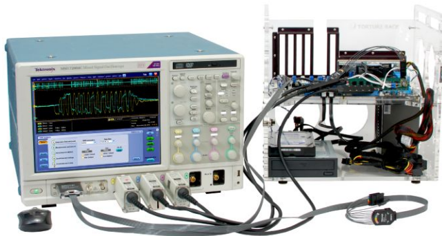
MSO70000 Series Oscilloscope probing command signals
