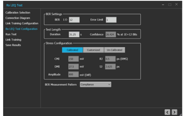
Tx-LEQ and Rx-LEQ test configuration
