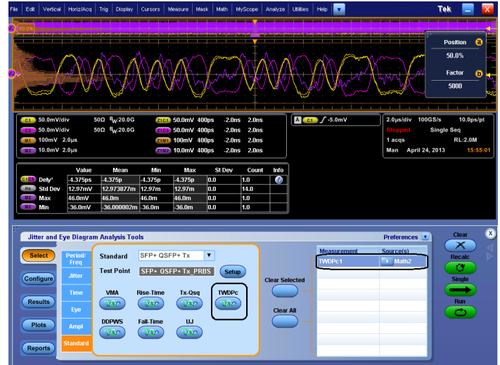
SFP-TX TWDPc measurement – DPOJET user interface.
