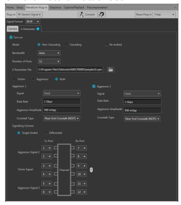
The Tektronix S-Parameters license unlocks the S-Parameter feature available in several of the application plug-ins (available for the AWG70000A Series Arbitrary Waveform Generators or the SourceXpress® application software) adding the ability to apply S-Parameters directly onto a waveform.
