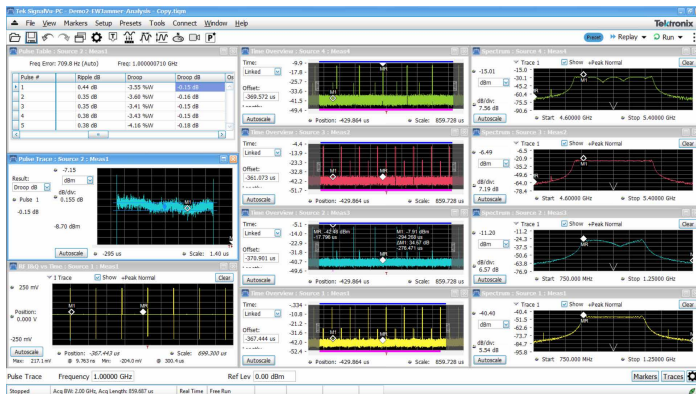
Four pulse trains are captured and analyzed simultaneously with time-correlated markers, pulse table, and pulse trace displays used to gain insight into the signal behavior across channels over time.
