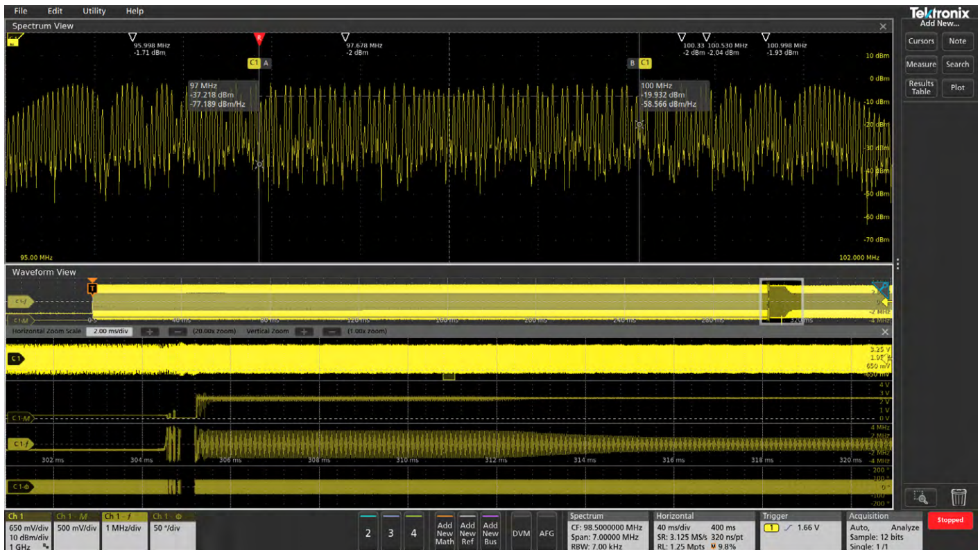
Figure 11. We've now zoomed in on the period of interest (roughly 300–320 ms after the trigger event). Notice that we can clearly see the amplitude fluctuating and the frequency changing over a broader range than it should be.
