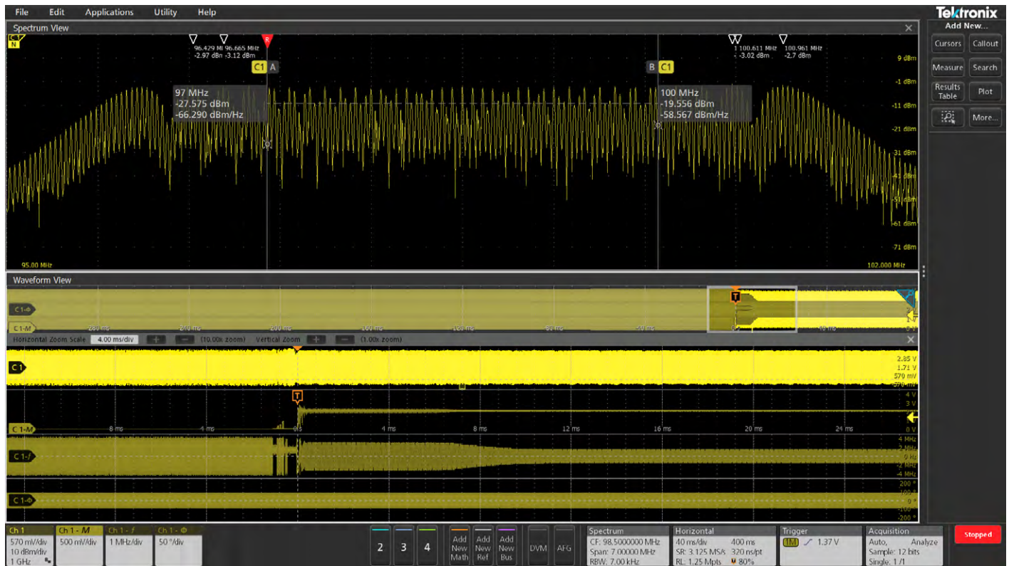
Figure 13. To focus on the clock turn-on, we can trigger on the RF magnitude waveform by specifying a threshold and edge using an RF vs Time Trigger setting. (Note: this measurement was made with more recent firmware than Figures 10–12.)
