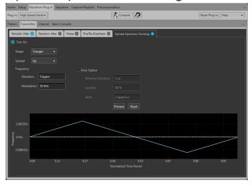
The Tektronix Spread Spectrum Clocking (SSC) license unlocks the SSC feature provided in the High Speed Serial application plug-in (available for the AWG70000A Series Arbitrary Waveform Generators or the SourceXpress® application software) adding the ability to add SSC modulation.
