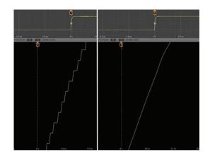
Figure 6: Zoomed in on a fast step, an 8-bit acquisition shows ADC quantization.
