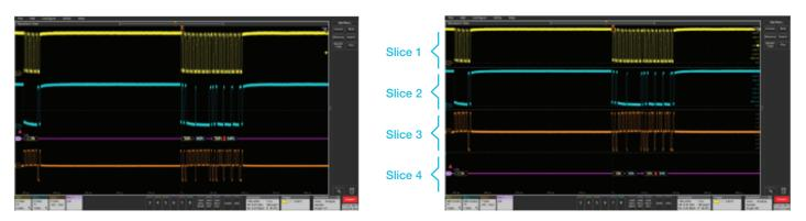
Figure 5: Each slice of the stacked display mode (right) can utilize the full range of the Tek049's ADCs, whereas each waveform in the overlay mode (left) uses only a fraction of ADC range.
