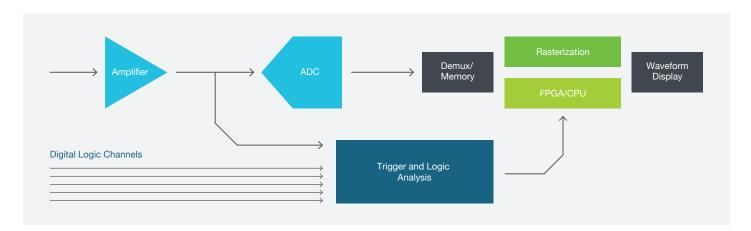
Figure 3 - Traditional oscilloscope acquisition path.
