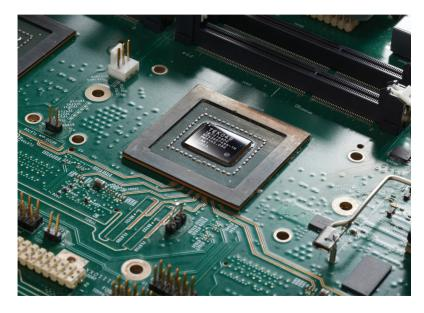
Figure 1 - The new Tek049 ASIC.
