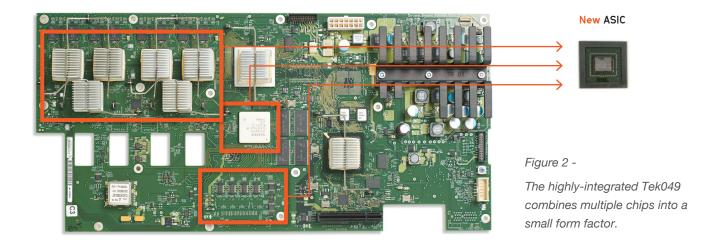
The new 12-bit ADC is the fastest in the world, running internally at 25 GS/s to give it a 25% higher sample rate per channel than previous oscilloscopes in its class. The 12 bits allow for 4096 vertical digitizing levels, providing 16x more resolution than other oscilloscopes utilizing 8-bit ADCs. Each ADC channel is based on an interleaved Successive Approximation Register (SAR) architecture, and each Tek049 chip includes four ADCs for a total throughput of 100 GS/s.
