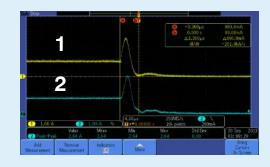
1=VCS5 Isolated Hall Effect Current Sensor 2=Tektronix TCP 312 probe w/TCPA300 Amplifier
